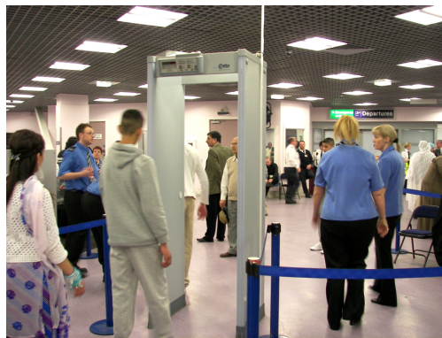
Figure 23.43 The familiar security gate at an airport can not only detect metals but also indicate their approximate height above the floor. (credit: Alexbuidrs, Wikimedia Commons)
